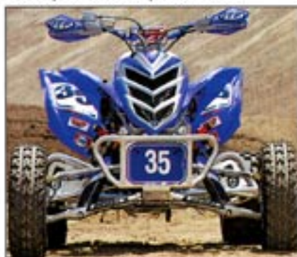
The Elka Elite Shocks, combined with the Laeger T-pin front end, give the front of the quad a very plush 13 inches of travel.
