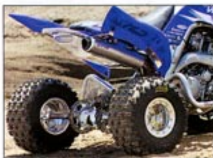
The rear end of the machine is equipped with Lonestar running gear, like axle, locknut and bearing carrier. The Elka Elite Shock and Golden West swingarm after a total of 10.5 inches of wheel travel.
